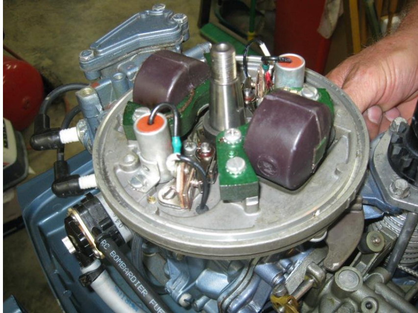
Kill wires attached to points sets and fed down through grommets in armature plate.
