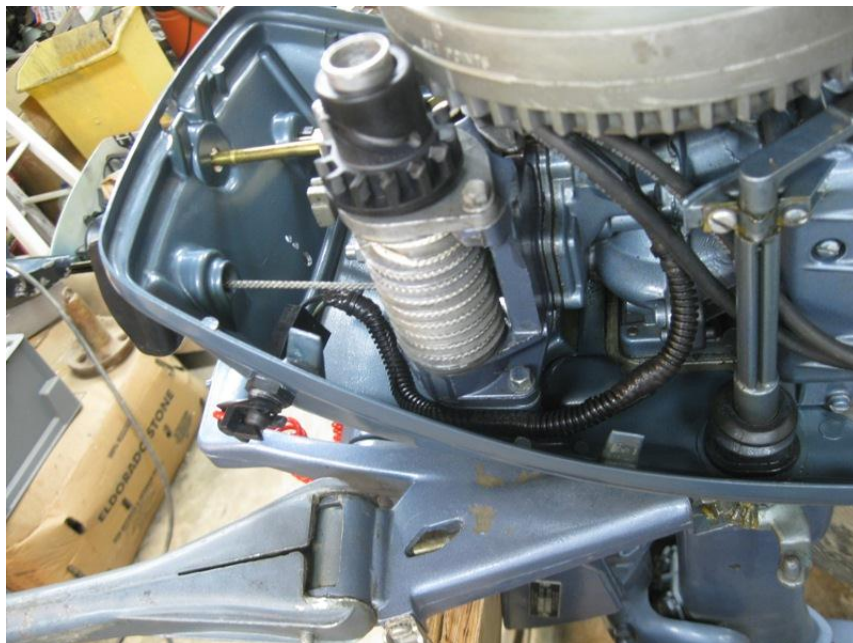
Kill switch wiring enclosed in wire loom from below flywheel to switch.
