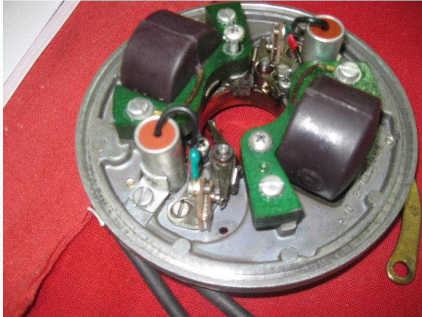
Small hole for kill wire at lower middle of armature plate.
