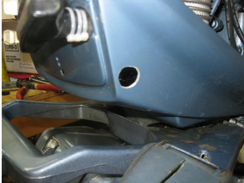
Hole for kill switch in an old, fantastically powerful, 6-hp Evinrude.
